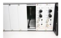
After mains and all other cabling have been removed, open the cover of a free slot in the ANC300. Carefully insert the module taking care not to touch the electronics with bare hands to avoid damages due to static electricity.
