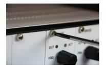
To open the housing, unscrew the two screws on the front side of the respective axis. The boards are connected to a backplate by a connector, so some force is required to pull them out. If possible, open a blank cover next to the module and hence get a better grip on the frontplate. Otherwise, use the BNC connectors (attach e.g. a T-piece) or the dials and carefully pull on them to withdraw the module.
