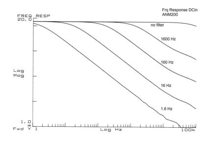
*Figure 12:* Frequency response of the ANM300 DC-IN input.
