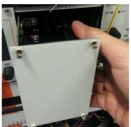
Pull out the power supply by grabbing the cooling body inside the ANC300. Do not pull on the frontplate!
