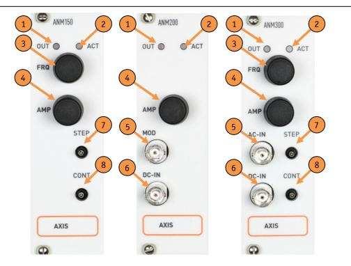
*Figure 2:* Front panel of the ANM150, ANM200 and ANM300 modules. The different items are explained in the text.
