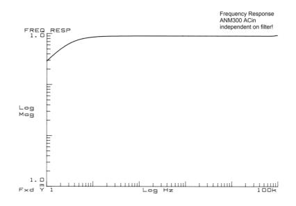
*Figure 7:* Frequency response of the ANM300 AC-IN input. Note that the gain is nearly 1 starting from a frequency of about 10 Hz and independent on the output filtering.
