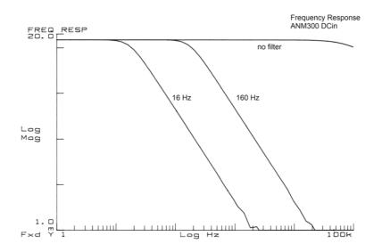
*Figure 6:* Frequency response of the ANM300 DC-IN input with different output filters applied. Note that the gain is 15 up to a frequency nearly up to 100 kHz. Note though that too high frequencies and amplitudes may damage the amplifier.
